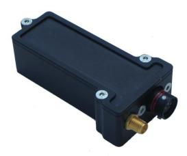
Compact, lightweight data receiver monitors RF signals from the TMS wheel transmitters. It decodes the sensor messages and sends calibrated pressure and temperature data to vehicle logging system via CAN or RS232 interface
