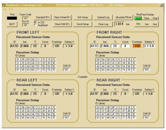
Allows modification of the sensor corner position library Setup of CAN message identifiers Enable/disable RS232 data output Enable/disable heartbeat function Upload/clear Receiver internal logging memory View individual sensor diagnostics
