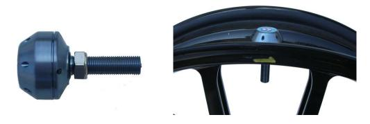
Measures and transmits tyre pressure and temperature, provides continuous monitoring of motorcycle tyres during test, practice and race conditions. Operates with TMS AS Receiver. Installs in a standard 8.8mm valve hole with O-ring seal as a valve replacement, accepts standard valve core. All valve threads conform to ISO 4570:2002
