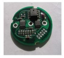
Latest development of the Brightwater TPMS motorsport sensor. Designed to transmit reliable and accurate tyre pressure data in an extreme operating environment.
