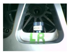
Measures and transmits tyre pressure and temperature, provides continuous monitoring of tyres during test, practice and race conditions. Operates with TMS AS Receiver. Installs in a 3/8" (9.5mm) fixing with a Dowty seal and K-nut. This sensor is compatible with the wheel hole used for the PI Research tyre sensor, widely used in Champ Car & IRL.
